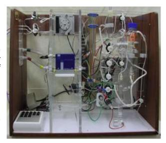
In principle, the VINDTA 3D is the DIC - part of the VINDTA 3C; see there for further details. The VINDTA 3D is prepared for the optional available separate **add-on units** for **gas calibration** with pure  $CO_2$  and for **salinity determination** from the same sample. Another option is a Peltier cooler option for the condenser (this saves one circulation bath).
